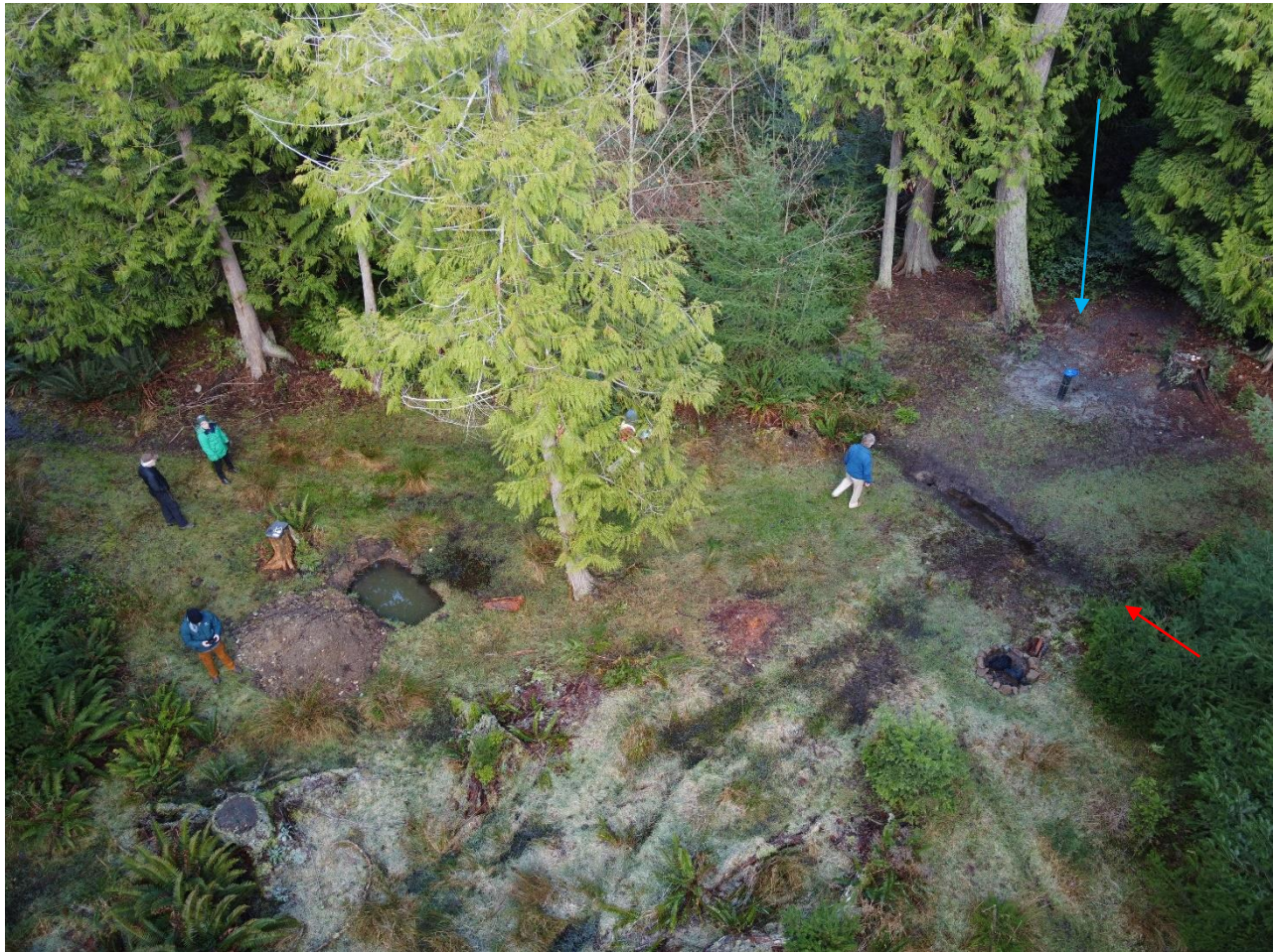
Figure 8. The ditch (red arrow) that crosses this open area near the well (blue arrow) would be disabled. The existing opening in the foreground would be used to build pond #1.
